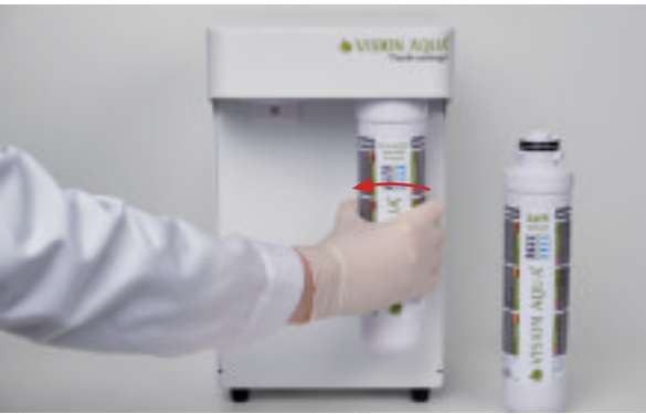
Turn the activated carbon post-filter unit counterclockwise 90° out of the filter head of the VA-Mini.
