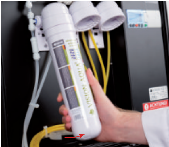
Thanks to the tilting filter heads, you can change the filter without additional tools. Take the GAC post-filter unit out of the Verdanium GEO in a forward direction.
