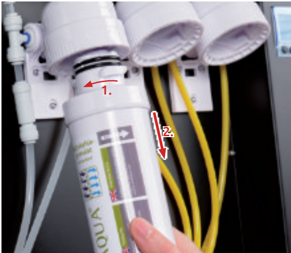
Turn filter cartridge counterclockwise 90° out of the filter head to change the filter unit.
