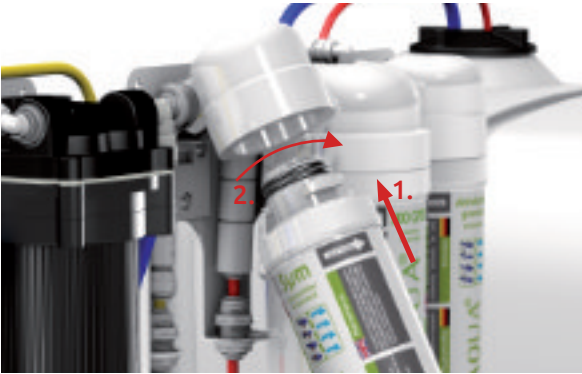
Insert the new filter cartridges into the filter heads, turning the filter cartridges clockwise by 90°. The filter units must then snap into the fastening clips.
