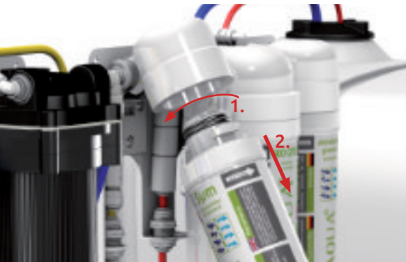
Turn the filter cartridges counterclockwise 90° out of the filter heads to change the filter units.
